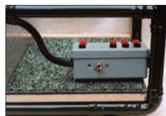
● Fig. 5: Make sure that the switch and wiring used has sufficient current carrying capacity for the total load you intend putting on the supply.
