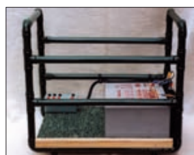
● Fig. 3: Made from easily available copper water pipe and fittings, the dimensions are cut to suit your needs.
