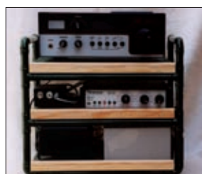
● Fig. 2: The final stage of making a copper pipe framework to carry the station for portable operations.
