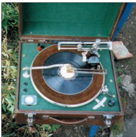
● Fig. 1: A portable disc cutting recording unit owned by John Gomer (see text).
